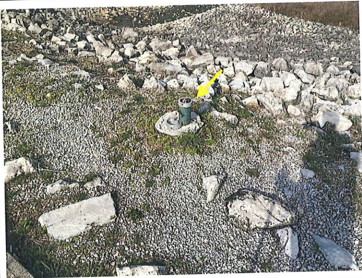
8. Downstream slope to the left of the principal spillway; arrow points to a piezometer.
