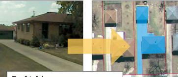
Roof + driveway = 3,000 sq. ft. impervious surface = 1 ERU
